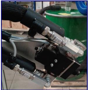
This combo system is designed for the pressing, gluing and rotation of wheels. It is controlled by a multifunction PLC with an operator panel that supervises all the working processes. This system is divided into two work stations: one for the flange gluing and pressing, the other for the core gluing during rotation .
